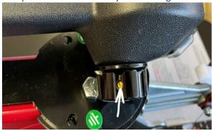
Remove the Hexagoanal nut as described and remove the potentiometer by passing it through the hole.
