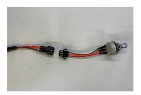
First perform a test by changing the potentiometer, only from the connector if your extension has one.
